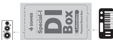
Keyboard → DI-box → Keyboard amp/mixer
